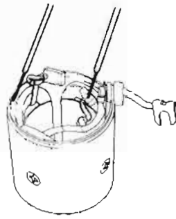
Fig. EE-17 Testing field coil for ground
